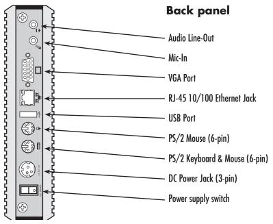
Figure 4. Ultra-Thin System - Back panel
